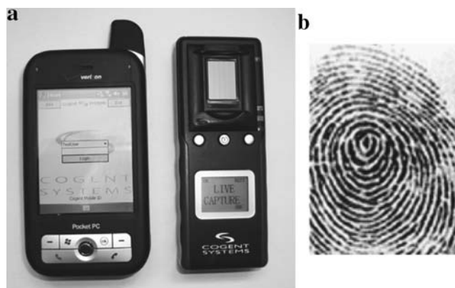
Fig. 1 a The Cogent BlueCheck™ handheld fingerprint capture unit with Bluetooth-enabled Verizon Pocket PC®. b An example of a right thumb print acquired from a living volunteer with a Cogent BlueCheck™ unit and displayed with NistViewer version 2.1 (Cogent Systems)
